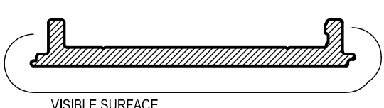
AD1024 BOTTOM TRACK BASE Mass. 0.636 Kg/m Anod. Per. 148 Paint Per. 100
